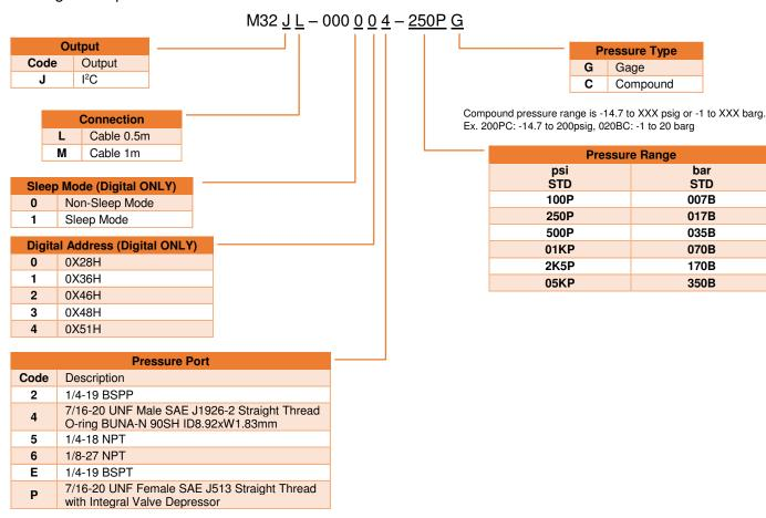
All Configurations are built with Voltage Reverse and Output Short-Circuit Protections. Click here for Torque Recommendation
