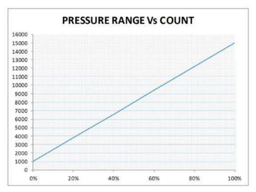
OUTPUT (DECIMAL COUNTS)=  $\frac{15000-1000}{\text{Pmax-Pmin}}X \text{ (Papplied-Pmin)+1000}$
