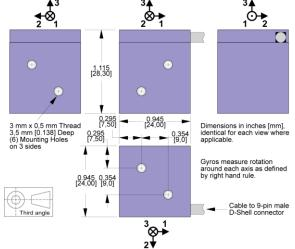
Two 3 mm x 0.5 mm threaded holes are provided on each of three orthogonal faces for mounting
