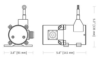
The PT8232 delivers position feedback via RS232 serial communication to your data acquisition or controller system. The PT8232 sends a raw 16-bit count from 0000H to FFFFH. Additionally this device can be set to continuously send data or send data only when polled.
