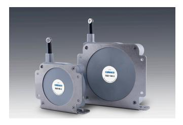
Suited for IP67 (wet) environments, the SGD provides a userselectable 4-20mA or 0-10VDC absolute linear position signal over an 80-inch or 120-inch full stroke range option. Signal selection is simply made by connecting the appropriate pins on the included connector or selecting the proper wires in the optional cordset.
