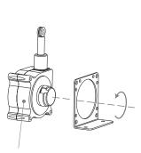
For added flexibilty, mounting bracket can easily be switched to the opposite side.
