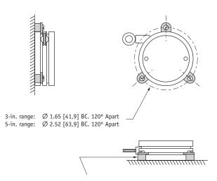
use 4-40 or M3 screws and servo-clips to mount sensor.
