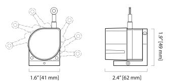
The MT3A is the solution for high-acceleration test applications in potentially wet environments. Just like the MT2A, the MT3A comes in 4 different full-stroke ranges, has a hightension heavy-duty measuring cable designed for the demands of flight and automotive crash tests and comes with an easy to use 2-axis 360° rotation mounting bracket for installation in hard to fit areas.
