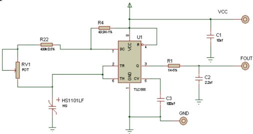
Note: R22=499k / R4=49.9k / R1=1 k / RV1=50 k potentiometer / C1=10nF / C2=2.2nF / C3=100nF
